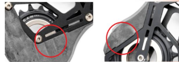
**!** Ensure that the clasps on the front and rear of the AERO COVER are flat against the front and rear plates.
