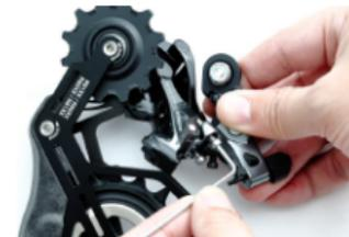
Some derailleurs may experience interference between the OPW and the derailleur body after installation. It is recommended to tighten the H bolt before installation to widen the derailleur body and prevent contact.
