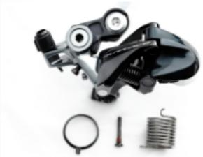
Remove the original derailleur cage and keep the original tension spring, axle fixing screw, and spring seal.
