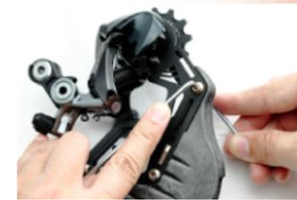
From the front end, gently push the Aero Cover into the OPW cage, insert the nut & bolt, then tighten them(max.4Nm) to complete the installation of the Aero Cover.
