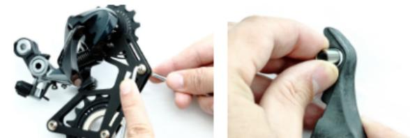
Using two 3mm hex keys to remove the plate nut, plate bolt, and bushing from front-end fixing hole.
