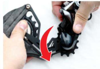
Rotate the outer plate counterclockwise until the fixing hole of the stopper pin is visible
