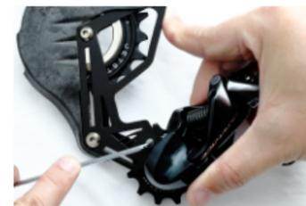
tighten the stopper pin using a 2.5mm hex key, then gently release the cage to reset, completing the installation.
