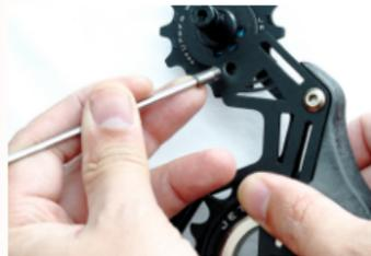
Remove stopper pin with 2.5mm hex key from TRiPEAK OPW cage.
