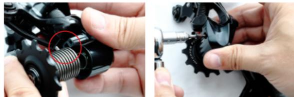
The spring stopper and seal should fit the tip into the mounting holes, then insert OPW cage's axle to derailleur body.
